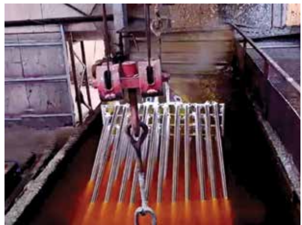
SCAFFOLDING HOT DIP GALVANISING
